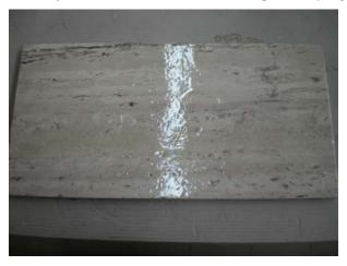
NOTE: the picture above shows an application of JOLLY - GLASS on travertine slab; see how pores keep perfectly visible. After polishing the results are surprising; the mastic remains transparent even in case of very thick coats.
